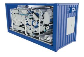
The **Dewatering or 'Beltpress' Unit** consists of an upper and a lower belt. The thickened sludge is processed through the rolls to further extract water which is then returned to the separation tank. The output of dry sludge cakes can then be transported away.
