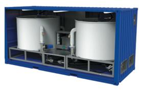
The **Sedimentation Unit** consists of two thickener units, which operate simultaneously. Pumps deliver sludge/water mix from the separation tank to the thickeners injecting an automatic dosage of polymers.
